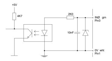
Picture 4: Synchronisation input INØ for TRIGGER measurement (see software manual)
