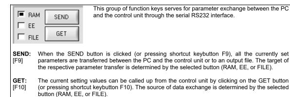
**RAM:** The current parameters are written to the RAM memory of the control unit, or they are read from the RAM, i.e. these parameters are lost again when the voltage is switched off at the control unit.
