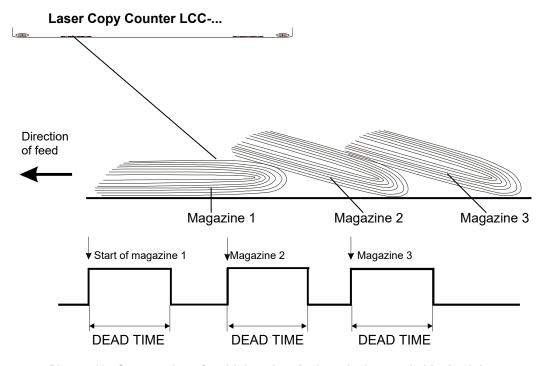
Picture 10: Suppression of multiple pulses by introducing a suitable dead time
