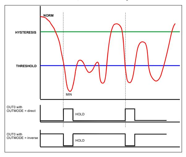
Picture 8: Measuring principle of edge detection
