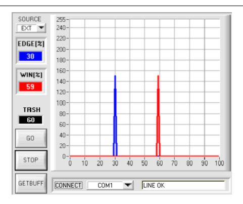
For operating the sensor with an active window, two initiators must inform the sensor about the active time. As described above, the active window is opened with a positive signal edge at input IN0 and is closed again with a positive signal edge at input IN1.
