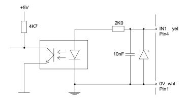
Picture 5: Synchronisation input IN1 for TRIGGER measurement (see software manual)
