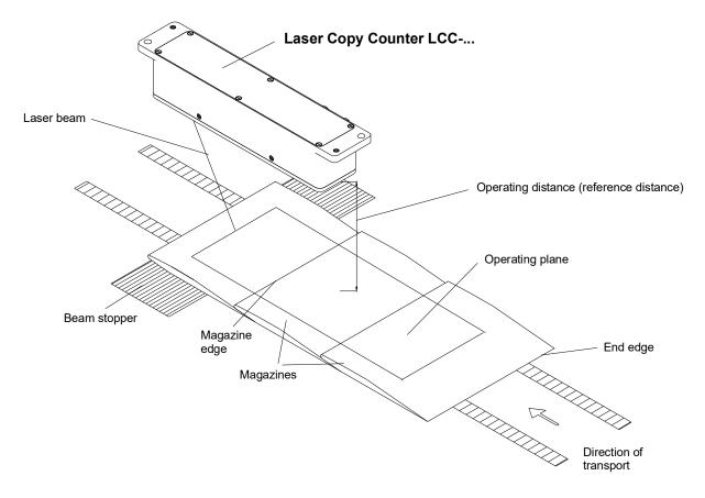
Picture 1: Application example for the Laser Copy Counter
